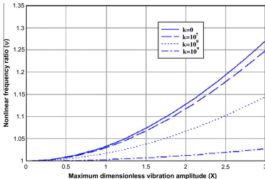
Fig. 3. Effect of spring constant  $k$  on nonlinear amplitude–frequency response curves of TWNT.
