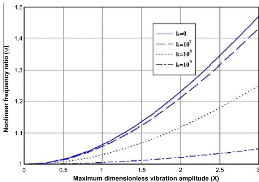
Fig. 2. Effect of spring constant  $k$  on nonlinear amplitude–frequency response curves of DWNT.
