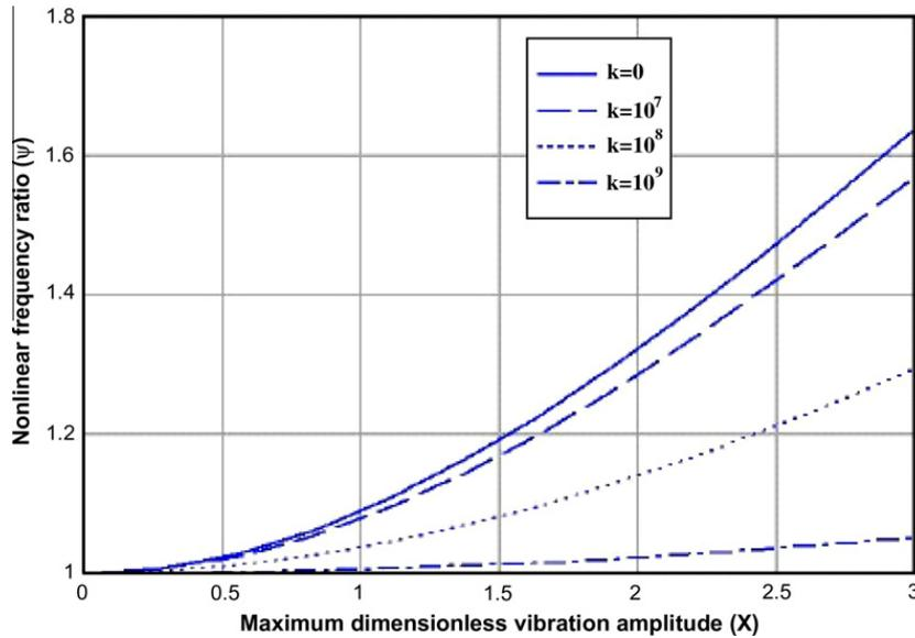
Fig. 1. Effect of spring constant  $k$  on nonlinear amplitude–frequency response curves of SWNT.
