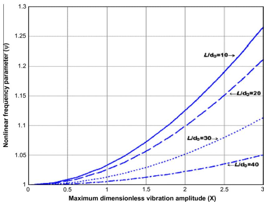
Fig. 5. Effect of aspect ratio  $L/d_2$  on nonlinear amplitude–frequency response curves for TWNT.
